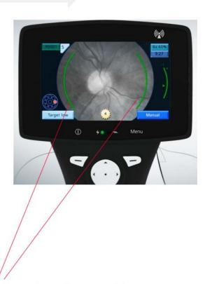
Carefully push the trigger when the two focussing aid lines turn from red to green Structures of the retina, e.g. optic disc and main blood vessels are visible depending on where the fixation target is set.
