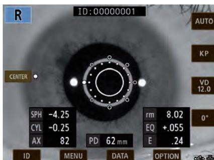
Corneal periphery measurement, eight points can be measured for the peripheral keratometry.
