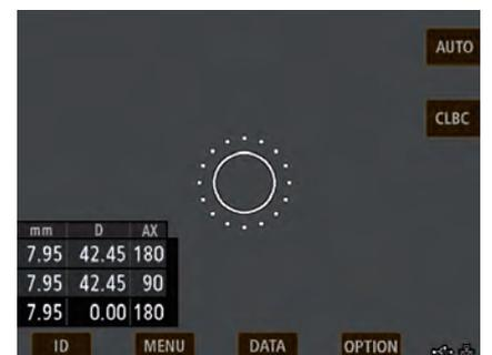
CLBC mode, useful for determining the base curve of a contact lens.
