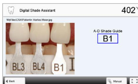
By double-clicking the touch screen, the image section can be enlarged and reduced again.
